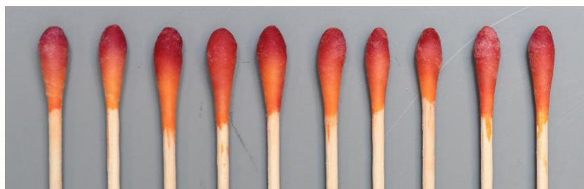
Figure 2. Reproducibility of the chromium-6 test at 5 µg chromium-6.
